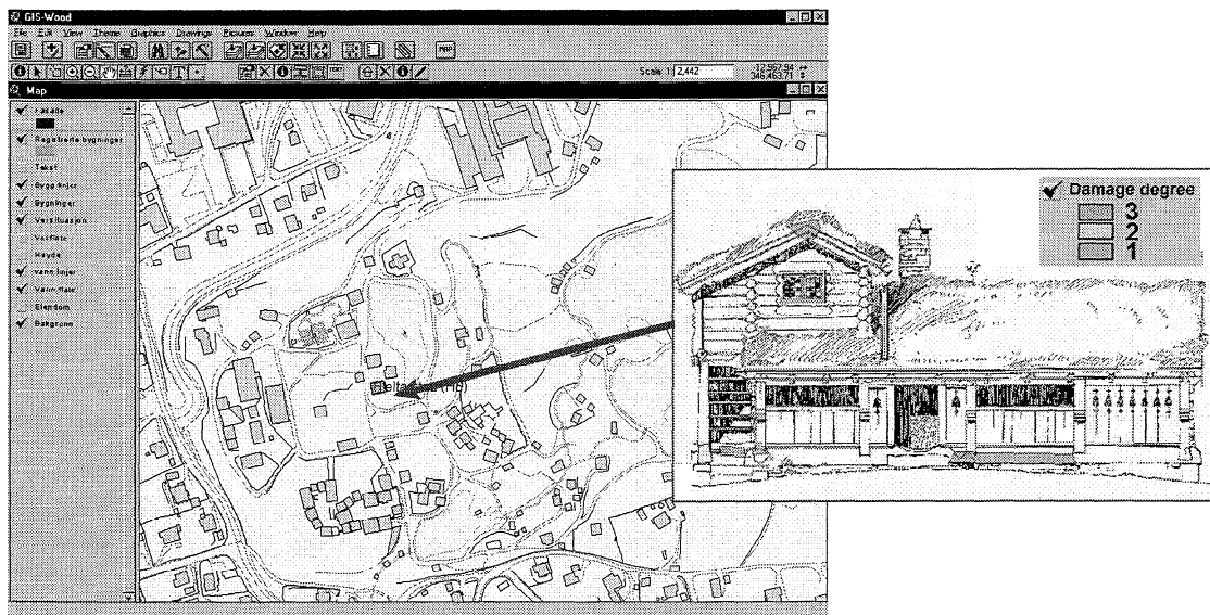
Fig 3 Damage assessment of Hjeltarstua at Maihaugen, Lillehammer exhibited in GISWood.
