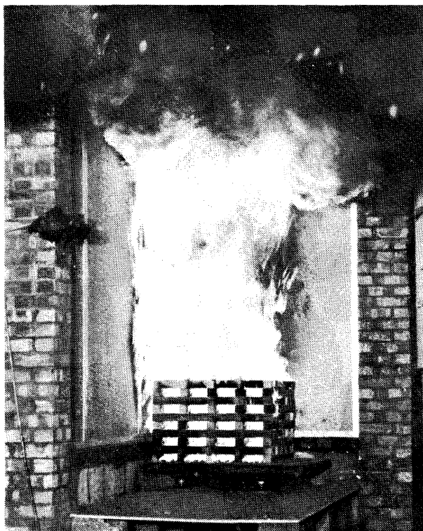
Figure 2 Corner-wall fire test in progress
