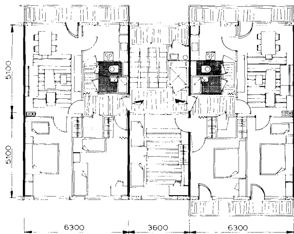
Fig. 1. Plan of dwellings built with large prefabricated panels and using a design based on long longitudinal interaxial distances.
