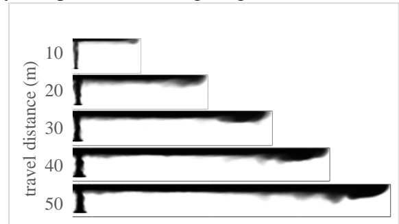
Figure 47: Evolution of ceiling jet bulb with travel distance of the ceiling jet (Figure shows half of the reservoir length)
