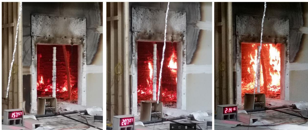
Fig 5: Regrowth of exposed CLT wall, 1 hr and 57mins through to 2hrs and 14mins into a compartment fire; from FPRF compartment fire test 1-5
