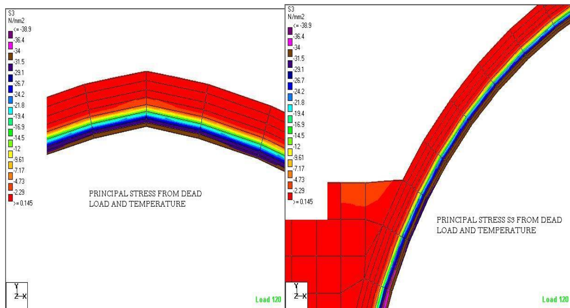
Figure 10. Solid stress contours on arches and buttresses from dead and thermally induced loads
