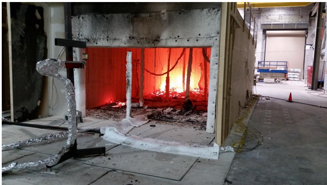
Fig 4: CLT compartment fire from the Fire Protection Research Foundation series of tests (undertaken by National Research Council, Canada with RISE, Sweden, at the National Institute of Standards and Technology)
