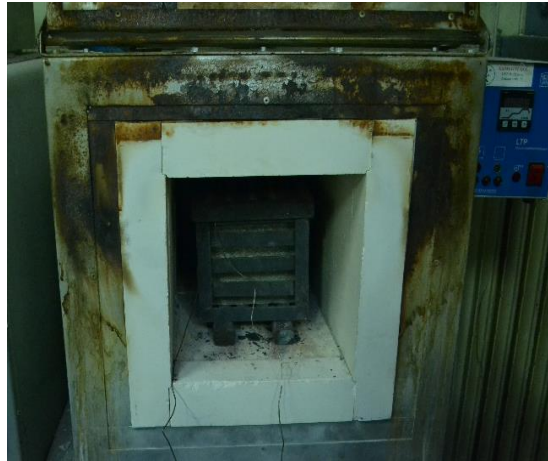
Figure 2: Electrical oven used in heating the specimens, showing the specimen covered by steel cage and two thermocouples from inside the oven to outside
