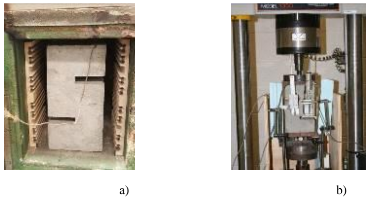
Fig. 4. a) Sample inside the furnace Hotpack for heating, b) Test setup for testing push-off specimen with LP for measuring vertical displacement.
