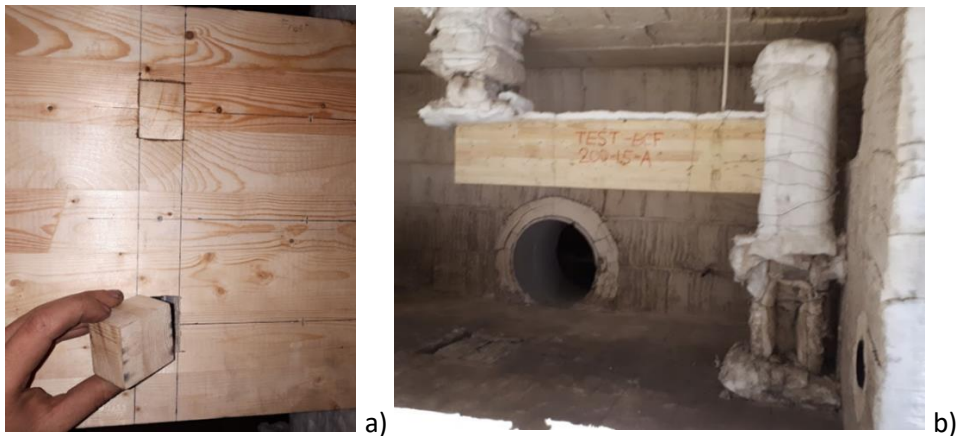
Fig. 3. a) Beam's side holes being plugged; b) A general fire resistance test setup
