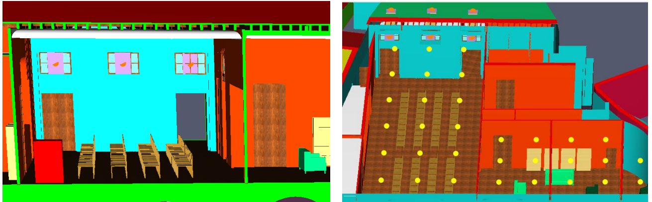
Fig. 5. View of the 3D model a) Scenario B, with exhaust fans b) Scenario D, with argon sprinklers
